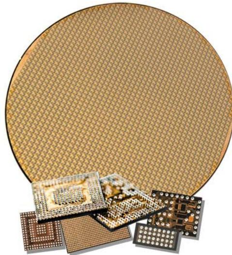
**Figure 1. eWLB panel after RDL and ball drop and eWLB samples**
